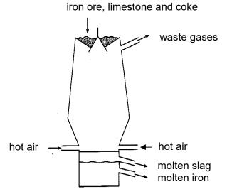
(a) Draw a line to link the raw material to its use in the blast furnace. [2]
