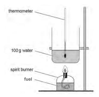
1 g of each fuel was used to heat 100 g of water. The results are shown below.
